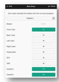
TIP: you can start a run-once program on the controller using buttons. This is useful for landscapers/gardeners to perform routine checks without having to give them WiFi access. To do so, press and hold button B3 until the LCD displays 'Run a Program'. Then click B3 to navigate through the list of available programs. Once you have found the program, press and hold B3 until the controller starts to run that program.
