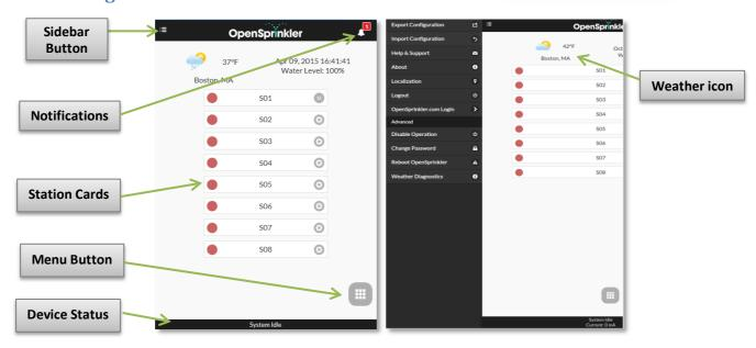
At the home page you will find a weather icon and list of all stations and their status. The bell button in the upper-right corner (when visible) indicates notifications are present and opens a sidebar with all notifications. The button on the upper-left corner activates the left sidebar, which shows additional menu items such as:
